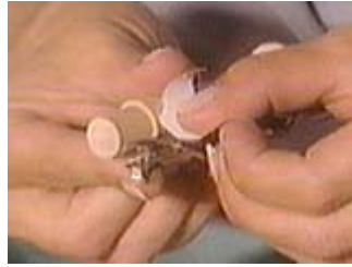
Mark the drill bit at the correct depth
