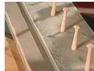
Use another board or straight edge to help mark for holes
