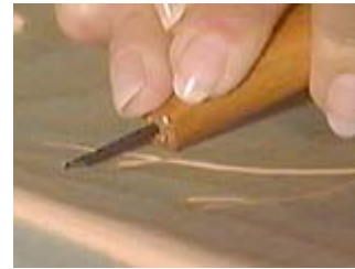
Carving using a micro v-groove carving tool for finer work
