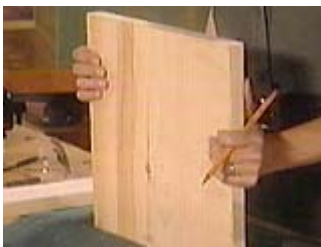
Be sure the wood grain in the legs is running vertically
