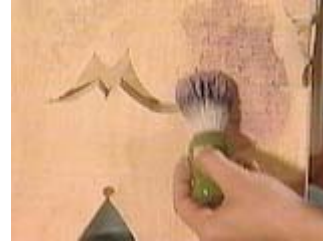
Apply the milk paint with a shaving brush
