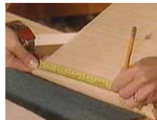
Mark the bottom of the 'V' three inches in from the edge
