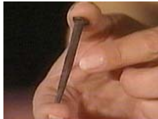
Reproduction nails are thick in the middle
