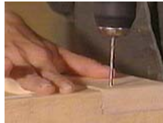
Drill for the nails
