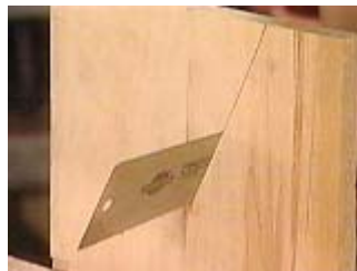
Cut out the v-notch creating the legs
