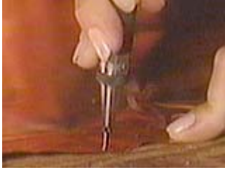
Use a compression punch to make dimples in the metal for drilling
