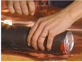
Use two soda pop cans taped together as a roller to bend the reflector into an arched shape
