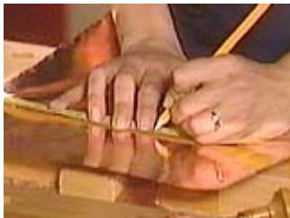
Mark the center of the reflector where you want the tabbed shelf to sit
