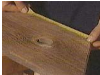
Measure and mark at six inches on the inside of the frame
