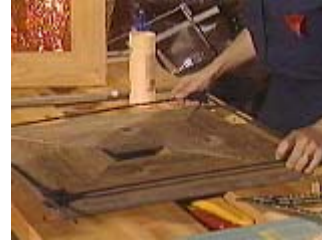
Place the frame clamp over the glued pieces and tighten it down
