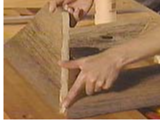
Use your finger to spread the glue around and remove any excess
