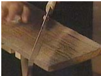
Use a Japanese style pull-saw to make the cuts
