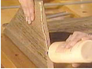
Apply glue to both sides of all the pieces that touch
