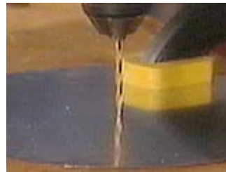
Use one or two more intermediate sizes to enlarge the dimple but don't go through
