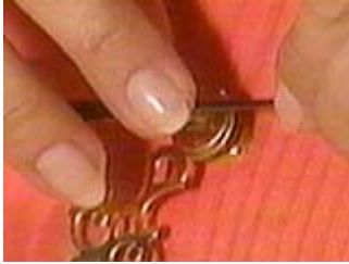
Press the second hand over the center pin on the shaft
