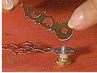
The minute hand is next and has a special slotted opening for the oval shaft
