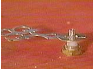
The hour hand goes on first and is pressed into place
