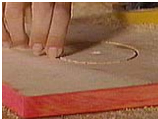
Use a piece of wire to test the depth of the hole saw cut
