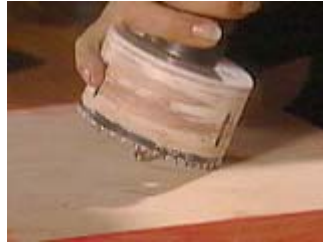
Place the pilot drill of the hole saw on the mark where the shaft will pass through
