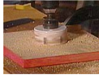
Cut a hole just deep enough to accept the clock mechanism
