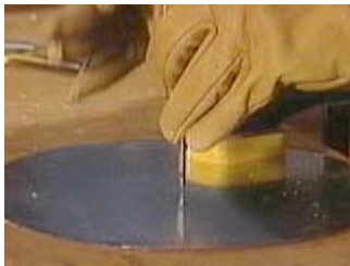
Use a nail or compression punch to make a dimple in the center
