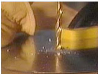
Finally, use a drill bit just larger than the shaft on the mechanism
