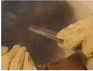
Use a file to clean up any burrs or sharp edges on the metal
