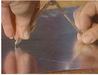
For a sheet metal face, scribe a cut line with a compass
