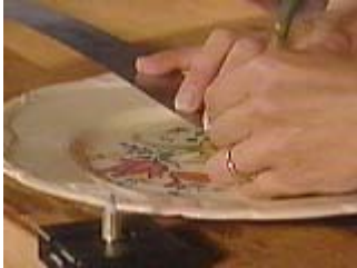
For a ceramic clock, mark the center point for drilling
