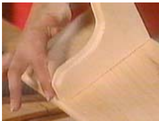
Use a scroll saw to cut brackets and a router to give the same edge as the shelf
