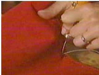
Push the sewing awl through the leather
