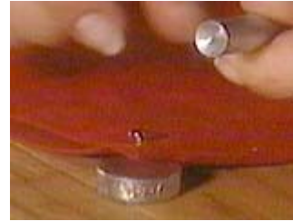
Concave end of hammer rivet setting tool
