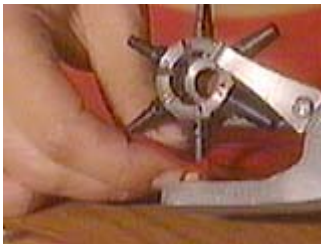
Use a leather punch to make a hole for the hammer rivet
