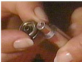
Female snap parts and setting tool
