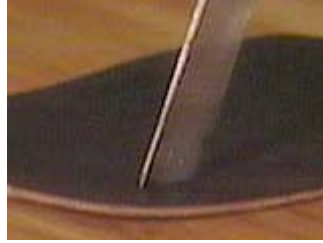
Cut out the slots for the belt with a chisel
