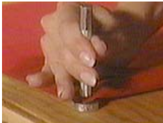
Place the concave end over the rivet and set it with the hammer
