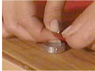
Push the post through the hole and place it on the baby anvil
