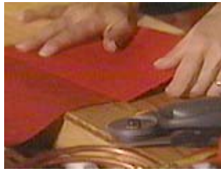
Fold the biggest piece one half inch out of square
