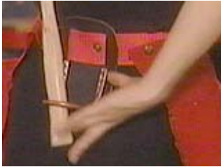
Hammer hook and belt in action
