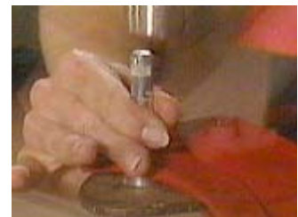
Setting the female snap on the leather
