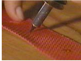
Use the hot iron to melt holes in the belt material
