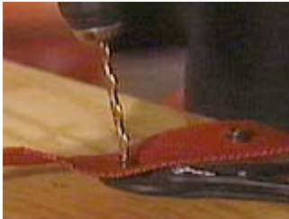
Removing an incorrect snap with pliers and drill
