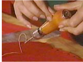
Pull the thread off the spool from inside the sewing awl
