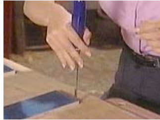
Hold the chisel like this for more stability
