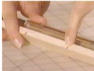
Measure and mark the jig at the drill points
