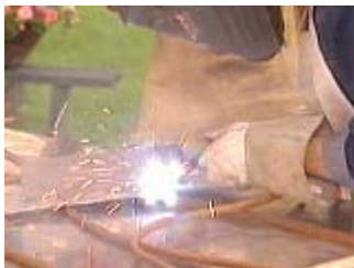
When the wire contacts the metal to be welded, the circuit is completed and the wire melts
