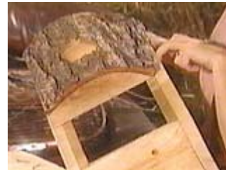
Attach little extender strips to the inside if necessary
