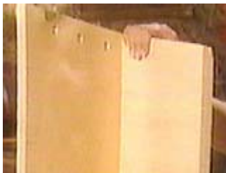
Drill ventilation holes and attach the side walls, back and floor
