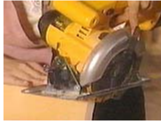
Adjust the saw blade to 15 degrees
