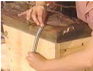
Attach the bottom 'trapdoor' section using a spring
