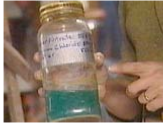
Copper nitrate solution used to create a blue green patina on copper
