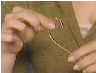
Form a hook with heavy copper wire
