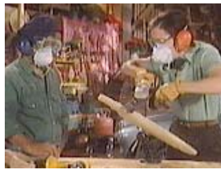
Use the Mini Grinder to scoop out the inside of the bowl
