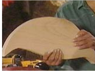
Use a jig saw or band saw to cut out the desired shape
