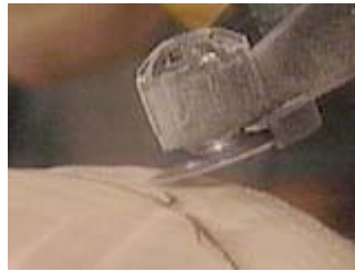
Use the Detail Mini Grinder for the fine work after the bulk of material has been removed
