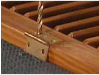
Drill off the heads of stripped screws
