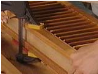
Clamp the 'sandwich' together and fasten with screws
