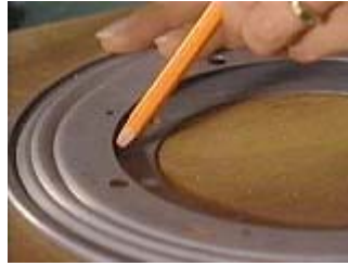
Center the lazy Susan on the bottom board and mark for the peep hole
