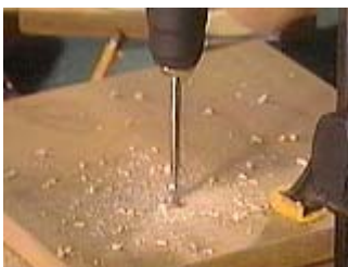
Drill a hole in the base the size of the peep hole
