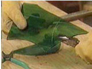
Use the breaking pliers to break along the line, down and away from the scored line
