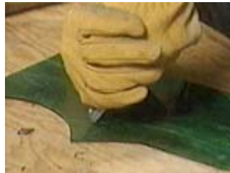
To cut the glass, press firmly while rolling the cutter over the glass
