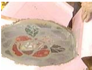
After it has cured for two or three hours, remove it from the form
