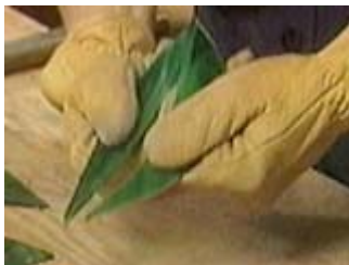
Use your gloved hands to break the glass down and away from the cut along the line
