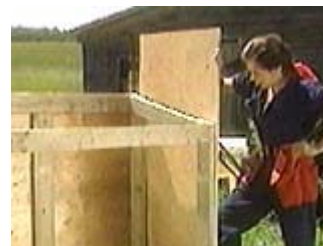
To mark the angle hold the plywood in place and mark
