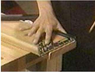
Check the end of the board for squareness and splits
