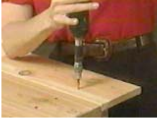
Pre-drill with a counter sink bit and attach the top boards
