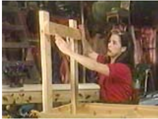
Install a horizontal support on the legs to hold a lower shelf
