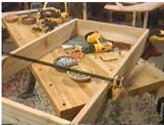
Clamp the apron or skirt frame together
