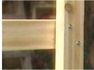
Attach the support with two staggered screws at each leg
