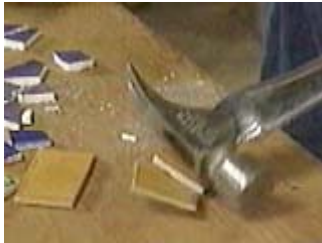
The easiest way to break tile is to hit it with a hammer
