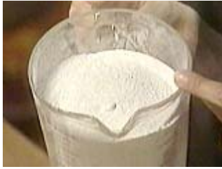
Use white 'Thinset' tile mortar
