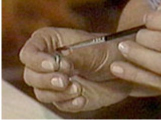
Brush shellac or nail polish on to the head of the screws
