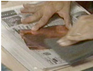
Treat the copper surface with synthetic steel wool
