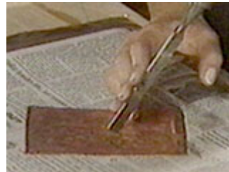
Use an old chisel to cut an X from corner to corner
