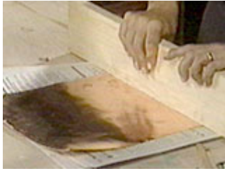
Place the scrap wood about half an inch in from the edge
