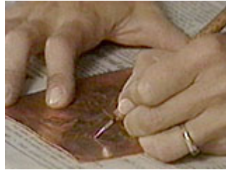
Use the ball end of the stylus to press the design into the metal
