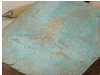
Five coats of vinegar first and then one coat of salt water
