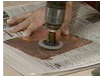
Synthetic steel wool also comes fixed to a mandrel which fits in a drill
