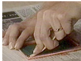
Use a Popsicle stick to press the copper against the switchplate
