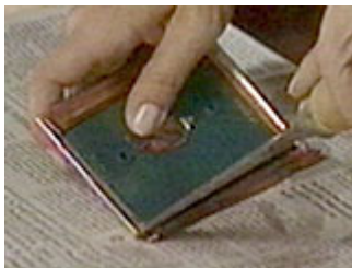
Use a dull chisel or straight screw driver to help make the corner folds
