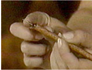
Stylus from an art supply store with punch end and ball end
