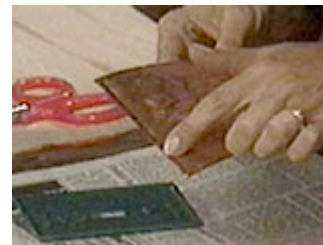
Option - Trim the sharp edges with sticky copper tape designed for use with stained glass
