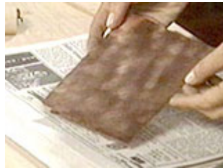
The surface looks like this after scrubbing with synthetic steel wool
