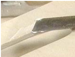
Fill any tear-outs or voids
