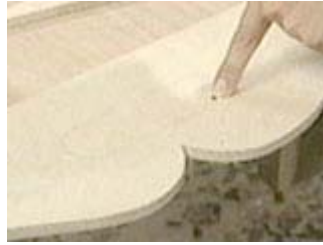
To cut out the handle, first drill a hole for the saw blade
