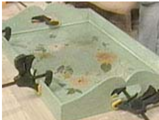
Cut and glue the trim in place
