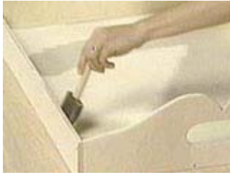
Apply the undercoat of paint first
