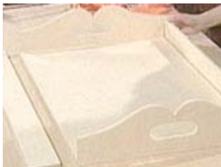
Dry fit the pieces and check for a tight fit
