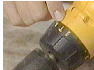
A drill with a 'hammer' setting makes cutting into rock easier
