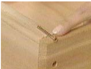
Use a screw long enough to get a good grip on the end grain
