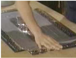
Tape the sides to the bottom
