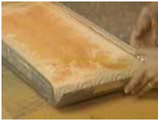
Peel the form away from the plaster
