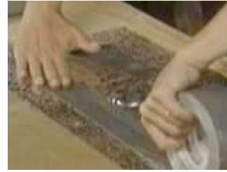
Tape the pieces together on the outside surface of the box
