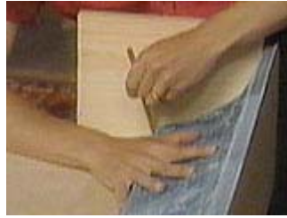
Mark the shape of the crown on a piece of pine
