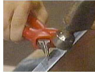
Hold the pins with needlenose pliers to start them
